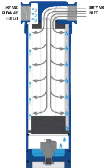
The Sullair range of compressed air filters is designed from the outset to meet current and forthcoming requirements for compressed air quality. Using aerospace technology, Sullair has optimized the flow path through the housing and element, significantly reducing air turbulence and pressure losses. Providing an optimal flow path is key to reducing pressure drop and system operating costs.
